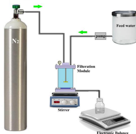
Fig. 1 The schematic of the used dead-end filtration.
